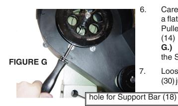
Carefully align both pulleys and tighten. Use a flat head screwdriver through the slot in the Pulley Cover (22) to tighten the Set Screw (14) on the Large Pulley (19). (See Figure G.) Use a hex key (not included) to tighten the Set Screw (14) on the Small Pulley (52).
